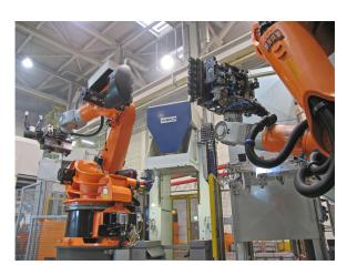
A relatively rare "hanging robot" Type KR500 is used in each of the casting cells in order to minimize the space requirements.
